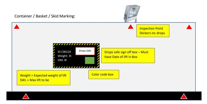
(Easy ID For Inspection – Does not cover the item in paint – Makes Drops on Containers, Baskets, Skids more apparent – Reduces the need for Container Drops lift checklist paperwork if the checklist is on the side of the container with highlighted areas – part of Drops / HSE Audit will be to renew stickers)
